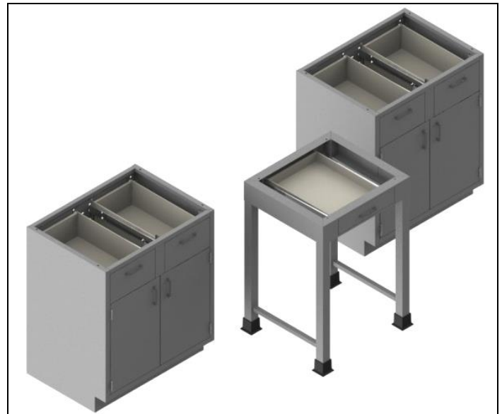
Step B: Move aprons and legs into position.
